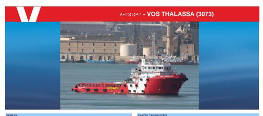
9606106 IMO Call Sign ICUE Place of Build Fuijan South East Shipvard, China Flag Italian Port of registry Vessel Type AHTS Year Built 2012 Class RINA Tug; supply vessel; anchor handling fire-fighting Class Notation ship - 1 -Oil Recovery ship - flash point > 60° C; water spraying; unrestricted navigation
